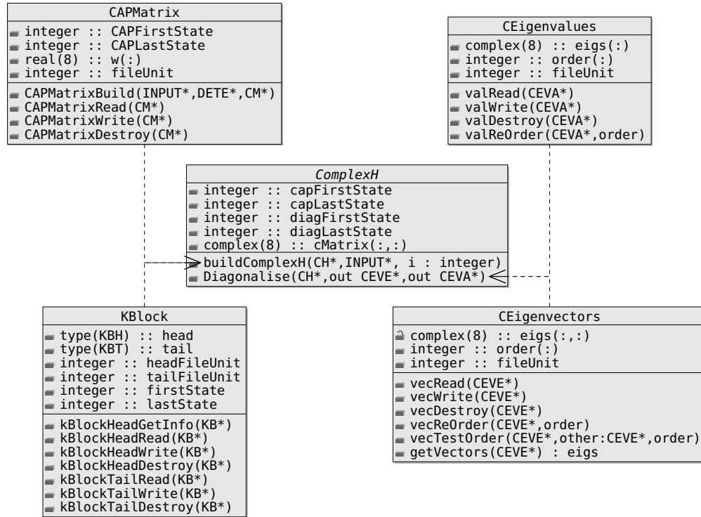
Figure 3.20: Class diagram representing the association of classes that lead directly to the construction of ComplexH objects. Only the public attributes and methods are displayed. All arguments in capitals with an asterisk are objects of the class with corresponding initials. The method buildComplexH() depends directly on the methods and attributes of CAPMatrix and KBlock and Input . The latter dependency is expressed through the declaration of an Input object as an argument of buildComplexH() . Note that ComplexH is an abstract class since it depends on external libraries such as LAPACK for the implementation of the buildComplexH() method.
