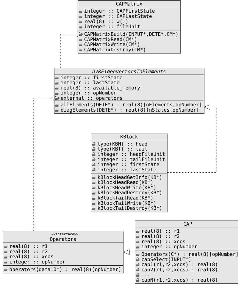
Figure 3.17: Class diagram representing the association of classes that lead directly to the construction of CAPMatrix objects. With the exception of class CAP only the public attributes and methods are displayed. All arguments in capitals with an asterisk are objects of the class with corresponding initials. The method CAPMatrixBuild() depends directly on the methods and attributes of DVREigenvectorsToElements and Input . The latter dependency is expressed through the declaration of an Input object as an argument of CAPMatrixBuild() . The interface required by DVREigenvectorsToElements for the operators() external function is defined by the interface class Operators and is realised by class CAP . The method capSelect() also depends on Input by passing its instantiation as an argument. The dependency of the methods of class DVREigenvectorsToElements on class KBlock is also illustrated.
